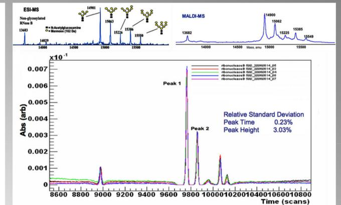
Ribonuclease B Glycoform analysis. Resolution of deltaDOT's data is comparable to mass spectrometry data
