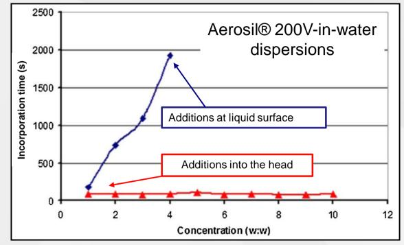
Ytron Y Jet: Powder addition into head constant rate of incorporation with increasing concentration
