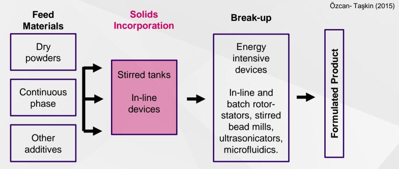
Typically 2 stage process, requiring incorporation into a stirred tank
