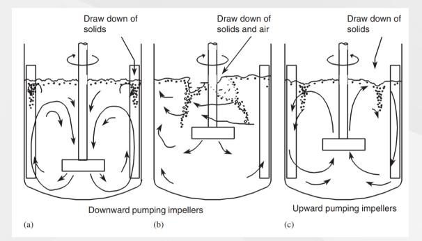
Powder incorporation in a stirred tank can cause particles to become trapped in dead zones, or result in air entrainment
