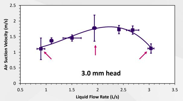
Incorporation time results could be explained with air velocity data at the powder inlet
