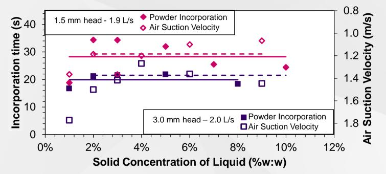
Incorporation rate with **3.0 mm** gap head was **faster** in line with the higher air velocities measured at a given liquid flow rate.
