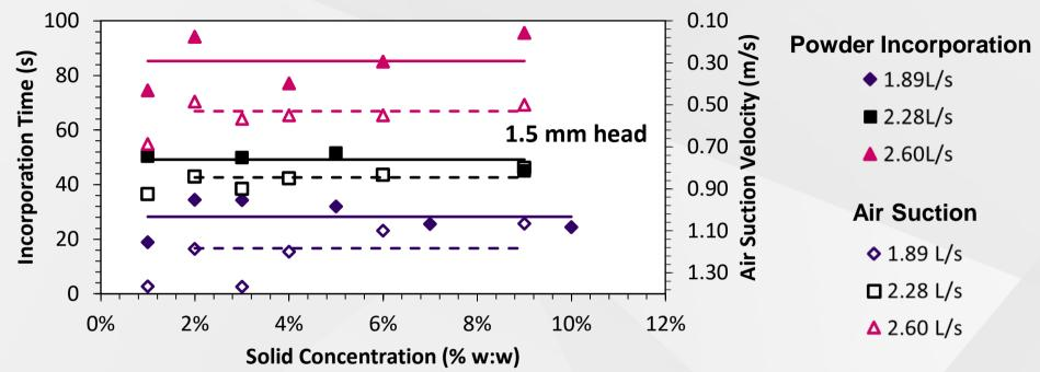
Air suction velocity at the powder inlet is indicative of powder incorporation rate
