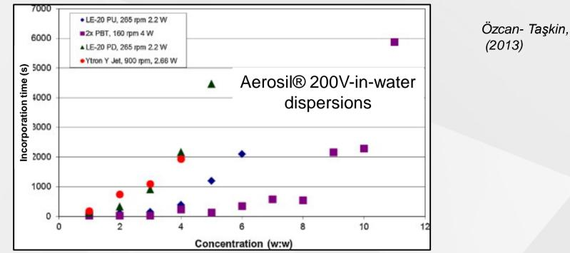
Additions at liquid surface (away from region of turbulence and fluid velocity) with a number of different impellers shows effect of solids concentration
