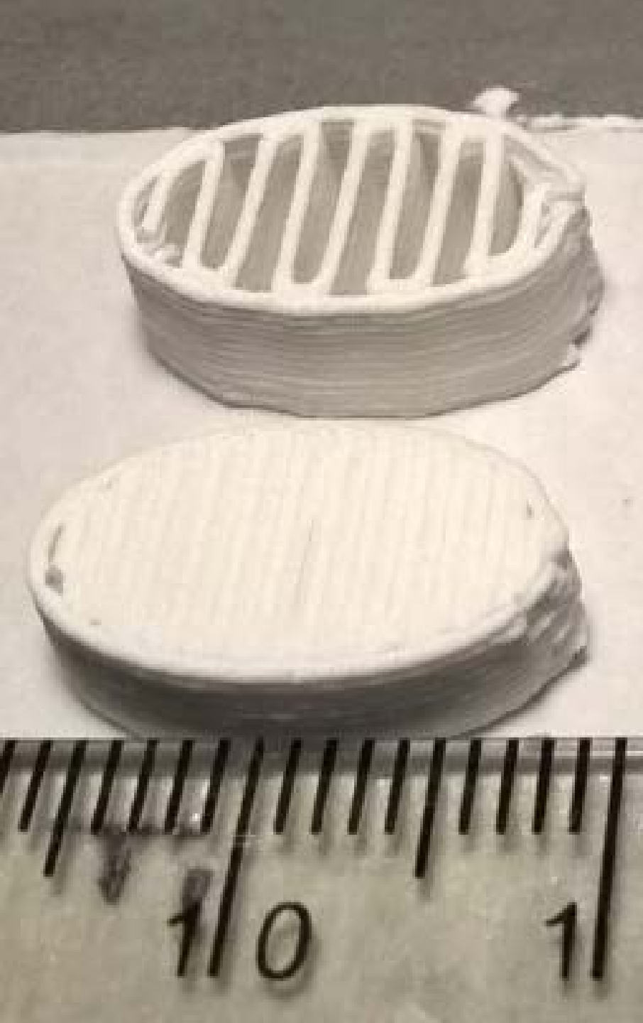
Extrusion 3D Printing of Paracetamol Tablets from a Single Formulation with Tunable Release Profiles Through Control of Tablet Geometry, Khaled, et al AAPS PharmSciTech, 2018
