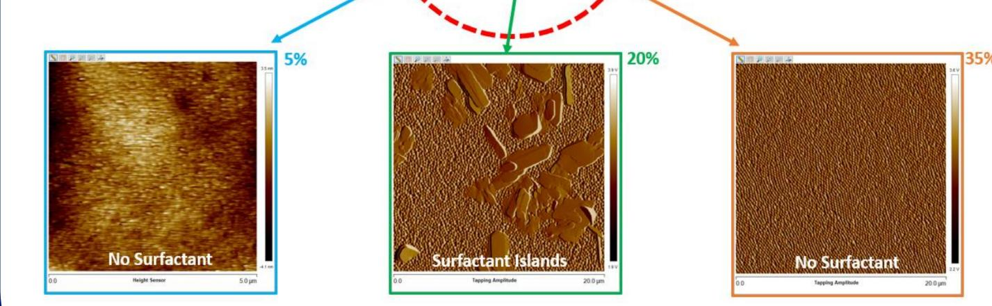
The results of the AFM appear to nicely confirm those from the RBS, agreeing that surfactant is only seen on the surface of films with an intermediate level of polymer cross-linking.
