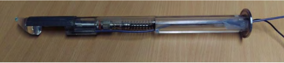
Probe with US and temperature sensor
